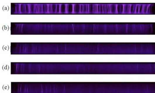
Fig.3 Discharges at different airflow speeds. (a) Flow speed v = 0 m/s, (b) v = 10 m/s, (c) v = 35 m/s, (d) v = 50 m/s, and (e) v = 100 m/s. Exposure time is 1/1250 s
