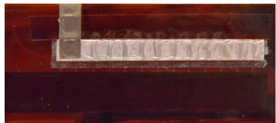
Figure 5. Comb-shape DBD actuator layout (Case 2).
