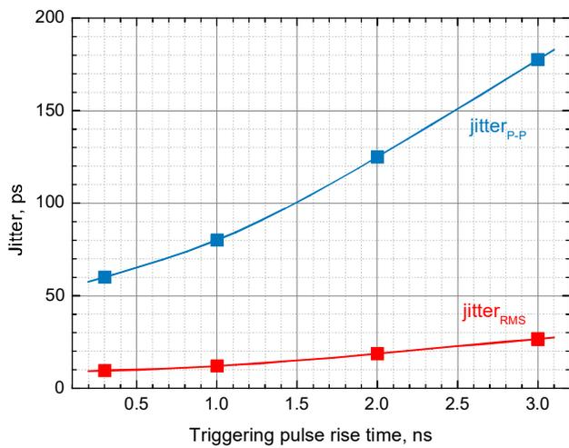
Fig.4. Output pulse jitter<sub>RMS</sub> and jitter<sub>P-P</sub> VS triggering pulse front rise time.
