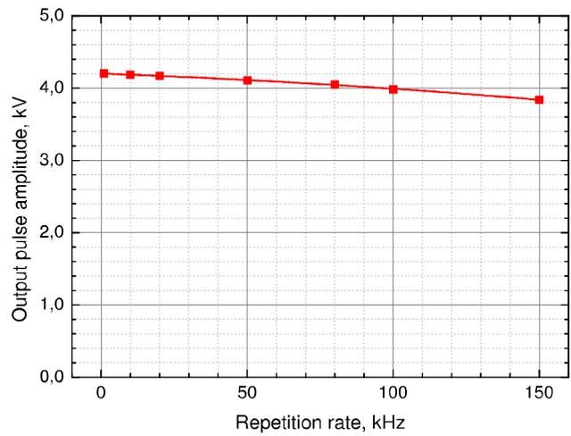
Fig.3. The typical dependence of the output pulse amplitude from repetition rate.
