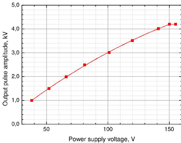
Fig.2. The typical dependence of the output pulse amplitude from high voltage DC power supply.
