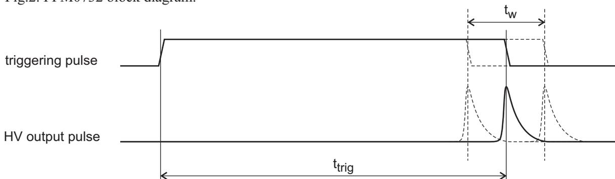
Fig.3. The timing diagram of HV output pulse synchronization with the trailing edge of the triggering pulse.
