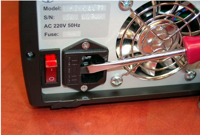
Fig.6. Removing of the fuse holder by flat screwdriver.
