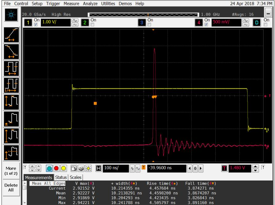
Fig.5. Oscillograms of SYNC OUT pulse (Channel 1, yellow line) and output HV pulse (Channel 4, magenta line).
