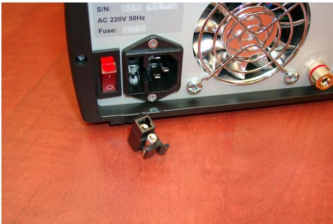
Fig.7. Two fuses in fuse holder including one spare (upper in the figure).
