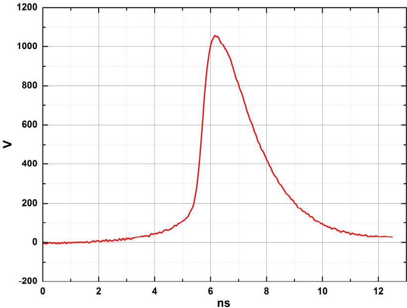
Fig.2. PPG-1/500 output pulse waveform.
