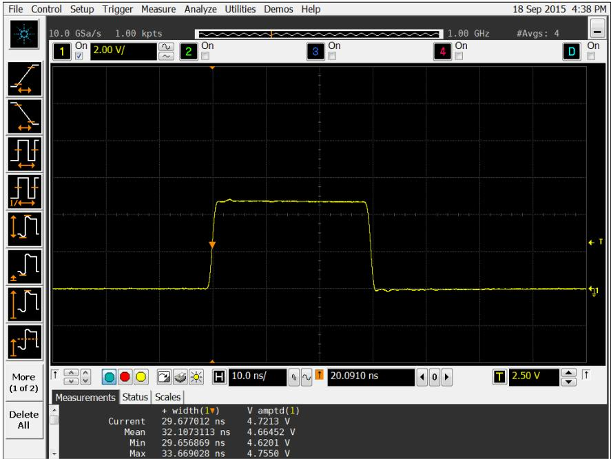
Fig. 5. Recommended triggering pulse waveform.
