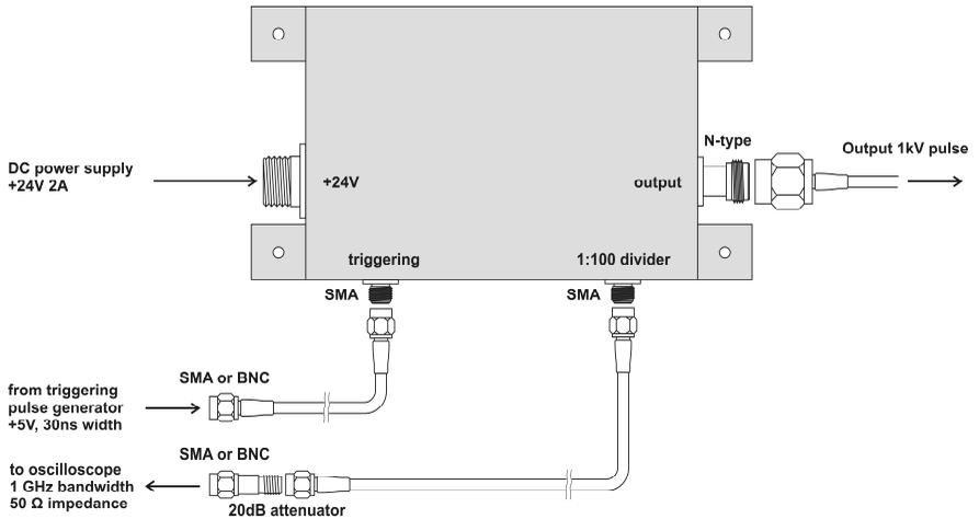
Fig.4. Connection of PPG-1/500 pulse generator module.
