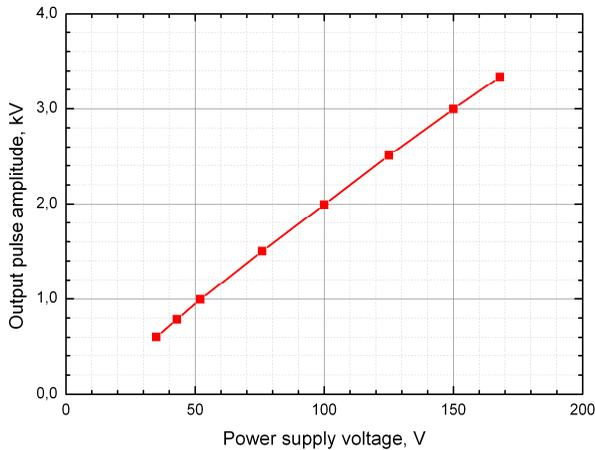
Fig.3. PPG-3/200 output pulse amplitude VS power supply voltage.
