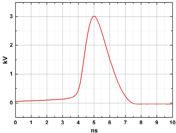
Fig.2. PPG-3/200 output pulse waveform.
