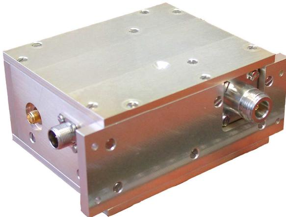
Fig.1. General view of picosecond pulse generator. The control LED are placed on the back side.
