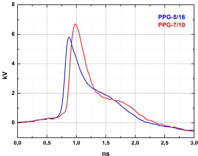
Fig.2. PPG-5/16 and PPG-7/10 typical output pulse waveforms.
