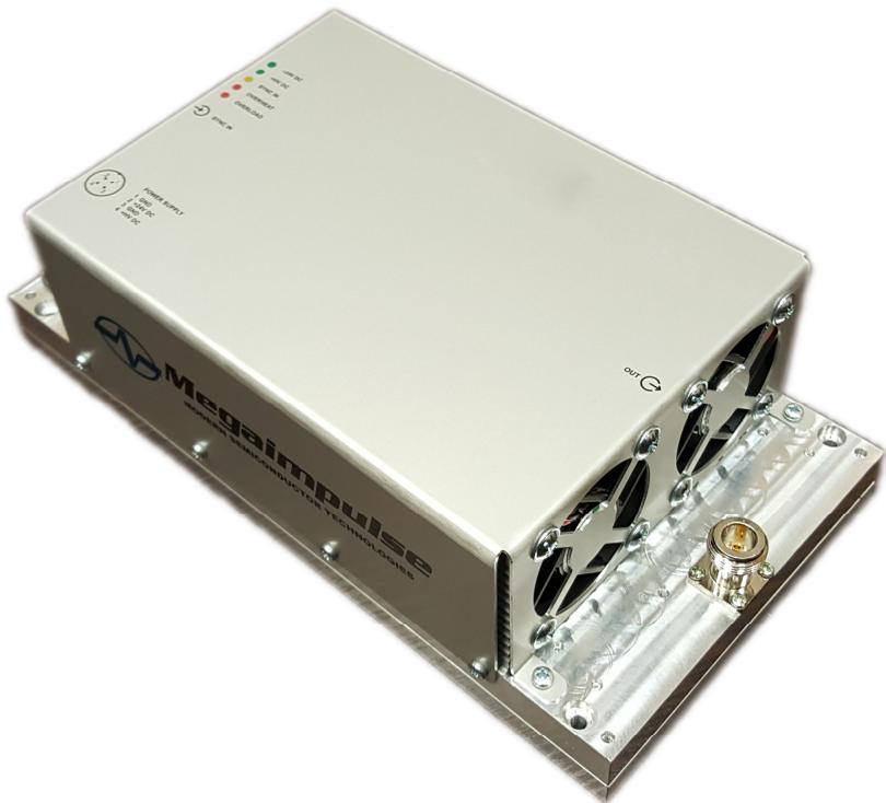
Fig.1. General view of PPM0531 picosecond pulse generator module.
