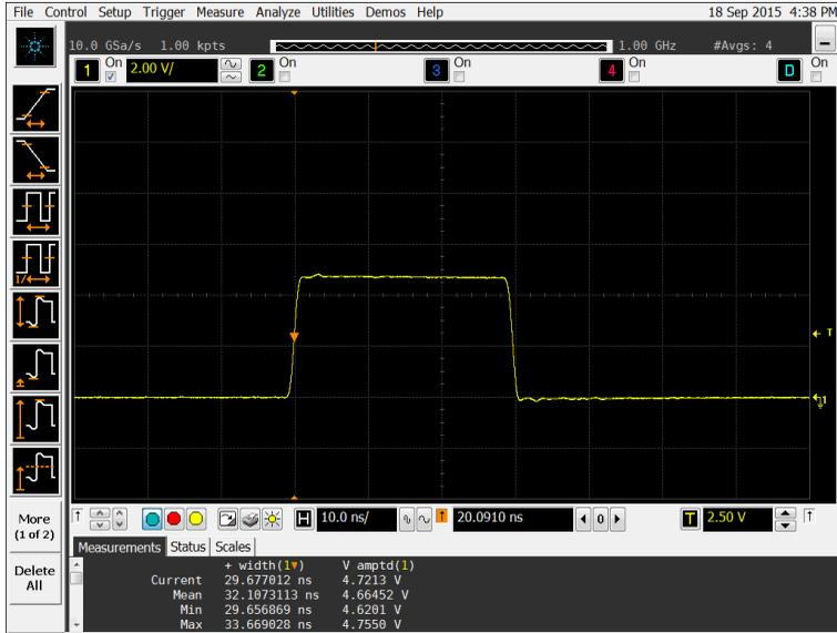
Fig. 5. Recommended triggering pulse waveform.
