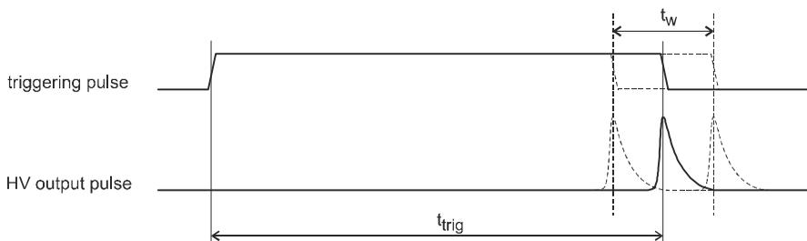
Fig.4. Operation of PPM0732 synchronization system.
